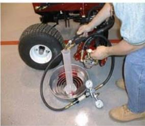
This measuring cylinder is used to measure flow on very low flow circuits. An example is measuring the flow from the case drain line of a hydraulic motor to test for motor efficiency.
