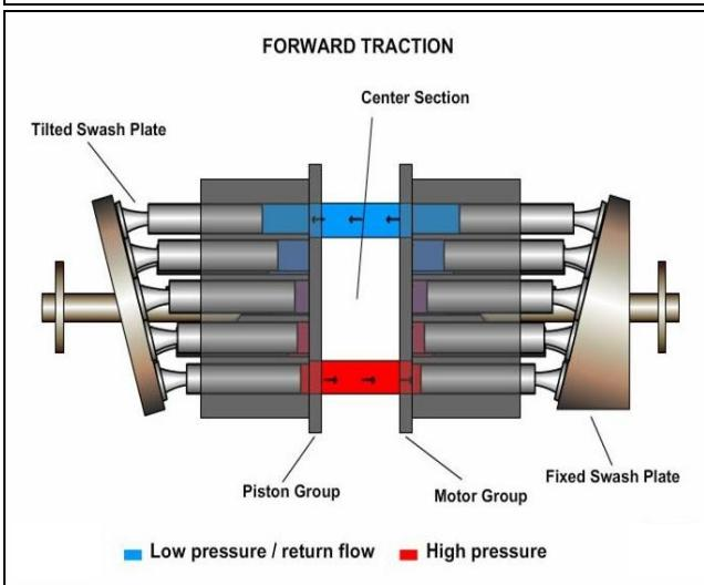
As the operator moves the traction control pedal the swash plate angle increases and the pump pistons begin to displace oil. This oil is directed to the pump section and the unit moves.
