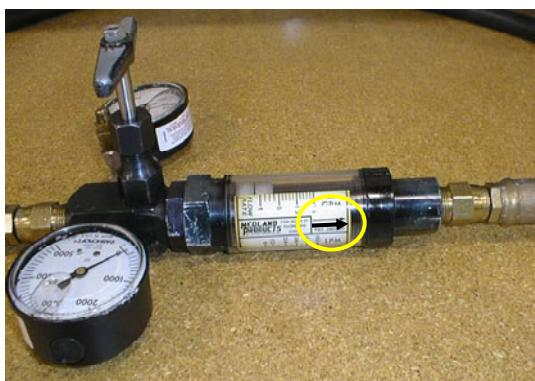
To prevent damage to the tester or components, the inlet and outlet hoses must be properly connected and not reversed (tester with pressure and flow capabilities).
