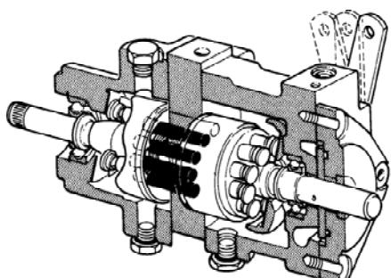
A different type of hydrostatic drive system is an inline pump and motor system. In this system the motor and pump are constructed as a single unit, this eliminates the necessity of high pressure drive lines between the pump and the motor. This unit is normally mounted to a drive axle or transaxle.
