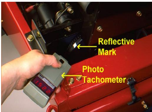
The engine must be in good operating condition. Always use a tachometer when doing a hydraulic test. ENGINE SPEED WILL AFFECT THE ACCURACY OF THE TESTER READINGS.
