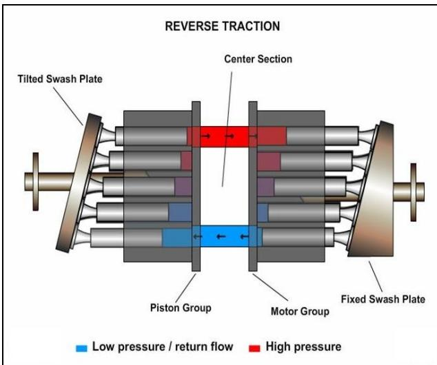
When the operator needs to change directions the traction pedal is moved back to the neutral position and then moved to the reverse position. In the reverse position the swash plate moves in the opposite direction as it did in the forward direction. In this position the oil is pumped to the opposite side of the motor and the unit moves in reverse.
