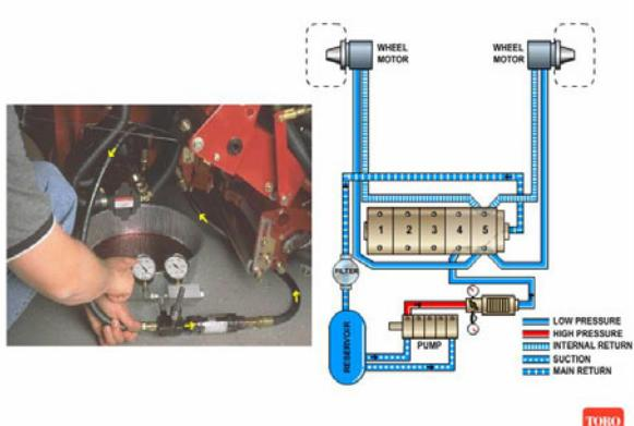
This is an example of a pump flow test. This test is also known as a pump efficiency test.
