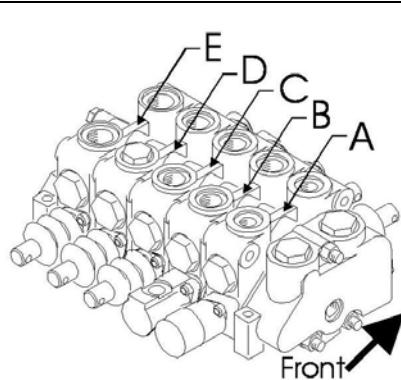
This is that same spool valve, assembled with multiple sections to make a valve bank or assembly. This example is from a Greensmaster riding mower. In this example the valve bank would control all of the hydraulic functions on the machine and would be actuated by foot or hand operated levers.
