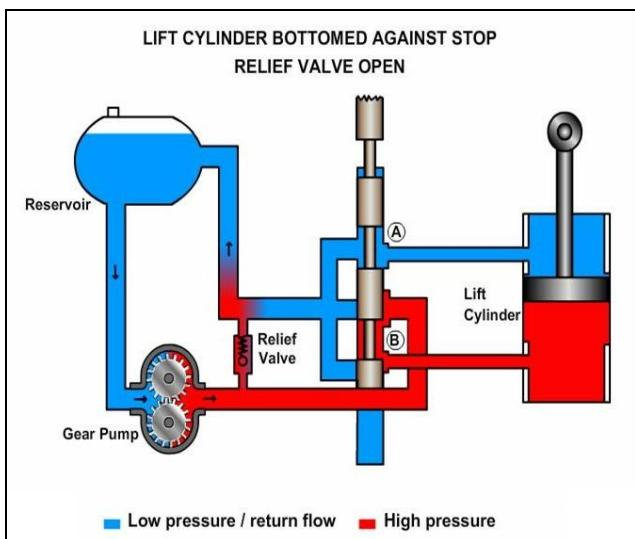
Since the fluid from a positive displacement pump must flow continuously whenever the pump is running, it must have some place to go if not being used by the actuators. If the load on the cylinder becomes too great or if the ram bottoms out, the flow from the pump will be directed past the relief valve returning to the reservoir.
