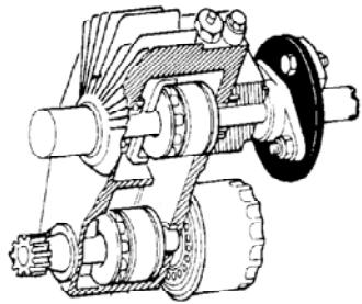
A similar version is the U-type transmission. In this type of system the pump and motor are constructed as a common component with the pump usually located above the motor.
