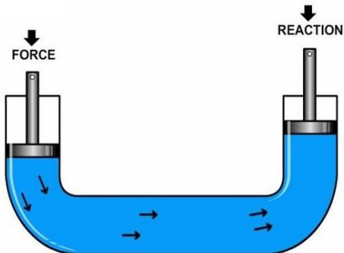
DOWNTWARD FORCE OF PISTON CAUSES OIL MOVEMENT OR FLOW IN THE TUBE
