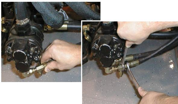
Install fittings finger tight, far enough to insure that they are not cross-threaded, before tightening them with a wrench.
