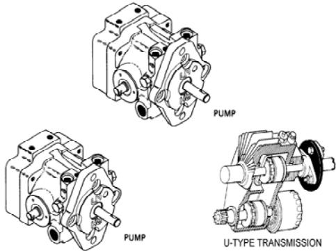
All three systems work well in their designed applications. The remote motor design works well when there is no transmission or transaxle, or when the location of the engine and the drive system call for such a configuration. The U type hydrostatic system is more compact while the inline hydrostatic system is usually easier to repair and maintain.
