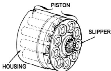
The pump consists of the following components:
