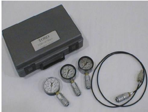
Hydraulic test equipment allows you to observe the amount of oil pressure and oil flow in a circuit under various conditions.
