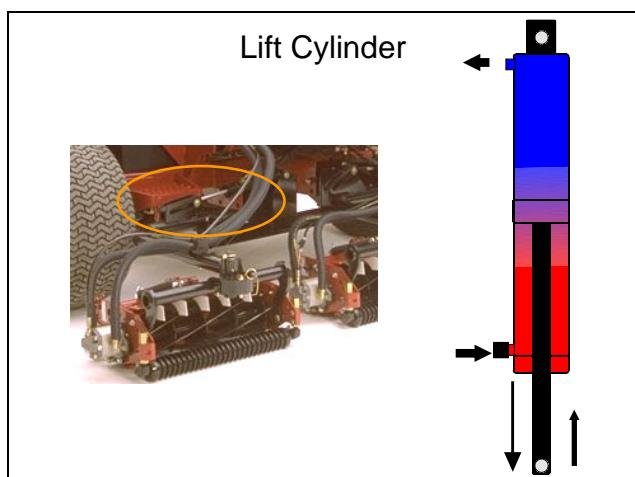
The flow diagram in the previous two illustrations shows the piston (barrel) end of the cylinder being pressurized to lift the load. Some lift circuits on Toro equipment pressurize the rod (ram) end of the cylinder to lift the load (e.g. Reelmaster 5000 series).
