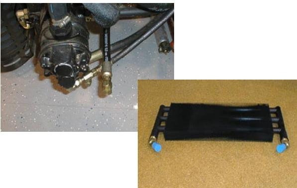
Put caps or plugs on any hydraulic lines left open or exposed during testing or removal of components.
