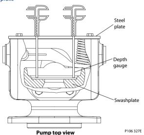
14. Hold the neutral return pivot in place using a 5/16 in internal hex wrench and tighten the seal nut using a 13 mm hex wrench. Torque seal nut to 22 N·m [16 lbf•ft].
