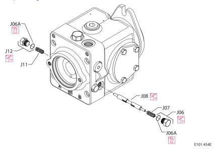
SYSTEM CHECK AND HPRV (HIGH PRESSURE RELIEF VALVE) Inspect plug and cartridge (M10,20). Inspect internal parts of cartridge (spring and poppet). If internal parts are worn or damaged, replace entire cartridge.
