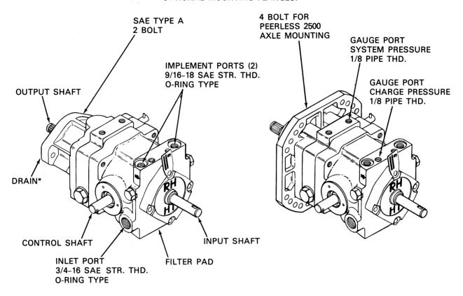
\* CASE MUST DRAIN DIRECTLY INTO OUTPUT AXLE OR GEARBOX THROUGH SHAFT BEARING.
