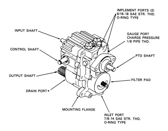
\* CASE MUST DRAIN DIRECTLY INTO OUTPUT AXLE OR GEARBOX THROUGH .406 DIA. PORT.
