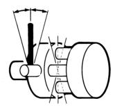
The speed at which the output shaft turns is proportional to the position of the control lever (or pedal) and is infinitely variable between zero and maximum speed. The direction of rotation of the output shaft depends on the position of the control lever (pedal) in relation to the neutral position (forward or reverse).
