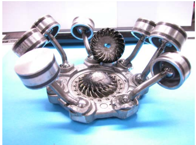
Overheated center ball and gear set
