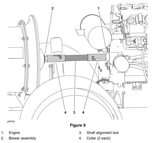
Align the engine output shaft with the blower shaft if the engine, blower drive shaft, or blower assembly is removed.
