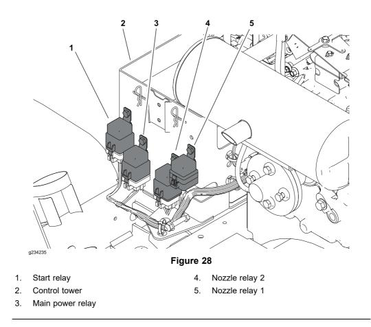
The electrical system of the Pro Force Debris Blower uses 4 identical electrical relays that have 5 terminals. A tag near the relay wire harness connector can be used to identify each relay.
