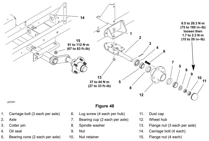
**Note:** Machines with Models 44552, 44552TE, and 44554 use an axle mount that is fastened to the frame. Machines with Model No. 44553 have a suspension axle for road ready machines. Wheel hub and bearing service is the same for all axle types.
