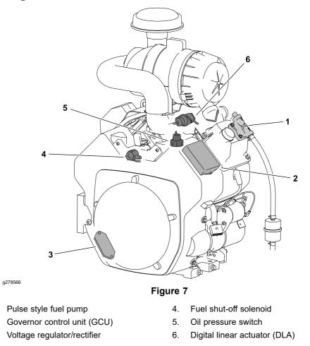
The engine includes an electronic speed control system. In addition to the necessary linkages, the speed control system includes a Governor Control Unit (GCU) and a Digital Linear Actuator (DLA). Electrical power must be available to the GCU for the engine to start and run. Engine speed is adjusted by using either the wireless or tethered remote. Refer to the KOHLER Command Pro CH740 Service Manual for additional information.
