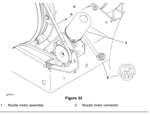
The motor used to rotate the nozzle is a reversible 12 VDC electric motor with an integrated gear box. The assembly components are not serviceable separately.
