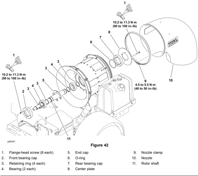
**Note:** The rotor shaft and bearings can be serviced without removing the inner housing from the machine.
