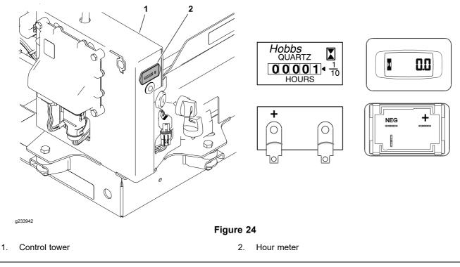
The hour meter used on the Pro Force Debris Blower records the amount of time that the engine is running.
