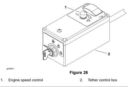
The engine speed control is a potentiometer located in the tether control box, and is used to control the engine speed (RPM).
