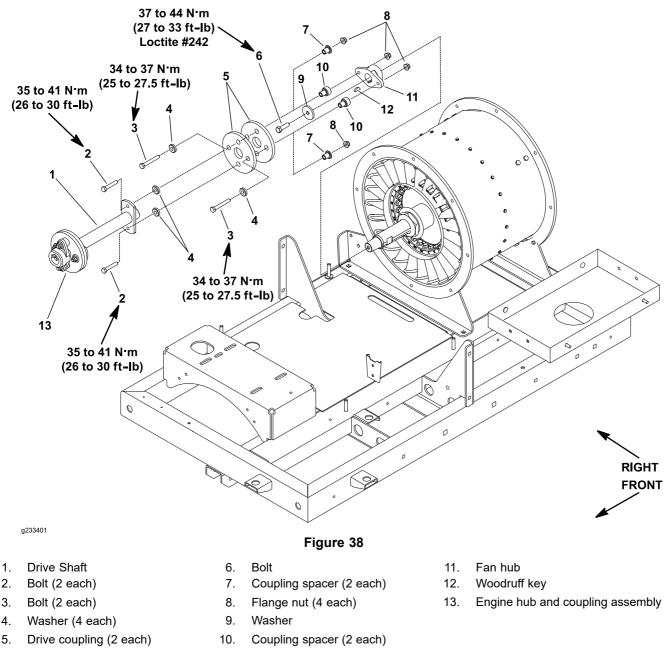
**Note:** The shaft hub and coupling assemblies used between the drive shaft and the engine shaft are comprised of the same components.
