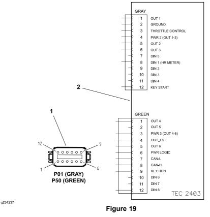
1. Wire harness connectors P01 (gray) and 2. Toro Electronic Controller (TEC) P50 (green)
