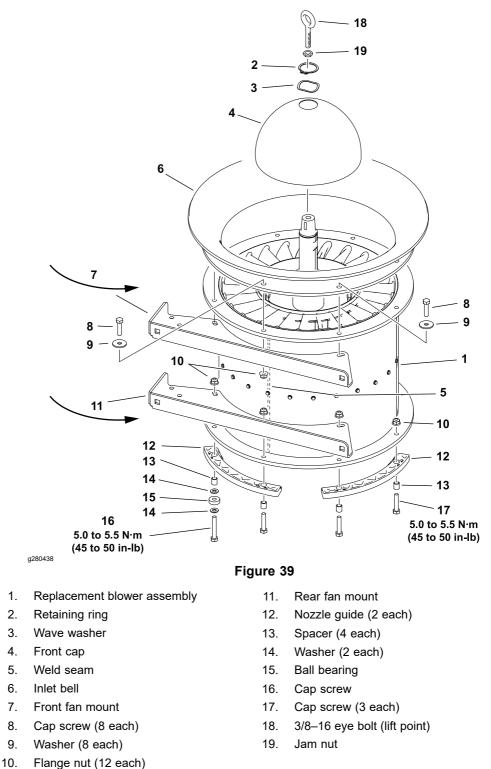
A replacement blower requires some assembly before the blower can be installed on the machine.
