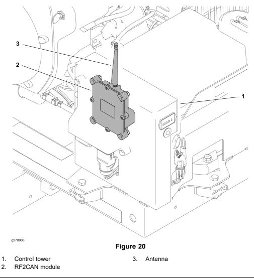
The RF2CAN module is a solid state electrical device used to convert radio frequency signals to and from the wireless handheld remote to CAN signals to and from the TEC. The RF2CAN module is only active when the key switch is in the RUN or START position. The RF2CAN module is mounted inside the machine control tower.
