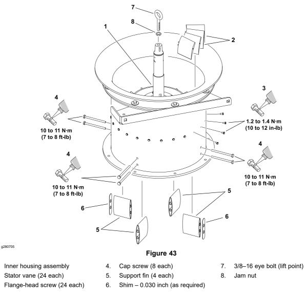
**Note:** The rotor shaft and bearings can be serviced without removing the inner housing from the blower assembly; refer to Rotor Shaft (page 6-10).
