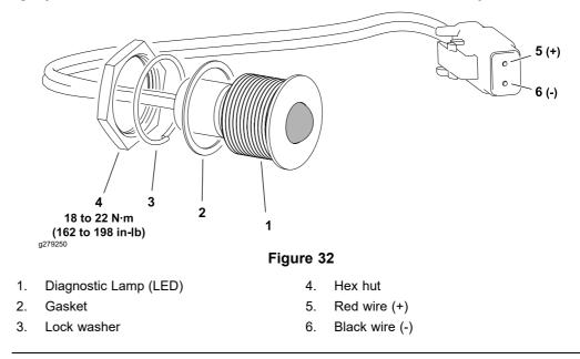
Machines with wireless remote control have an LED diagnostic light located on the machine control tower. The TEC controller uses the diagnostic light (output) to notify the operator or the service technician of an issue that may exist with the machine; refer to Using the Onboard Diagnostic Lamp (page 3–3).
