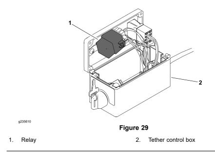
**Note:** Model 44554 machines have an additional 5 terminal relay located in the tethered control box. This relay is not presently being used.
