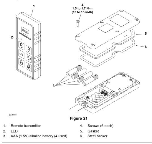
The handheld remote is a solid state electrical device that sends and receives radio frequency (RF) signals to and from the RF2CAN module. The handheld remote to RF2CAN module range should be approximately 4.6 m (15 ft). The handheld remote can only be associated to one specific RF2CAN module. Refer to the machine *Operator's Manual* for the handheld remote to RF2CAN (base) association procedure.
