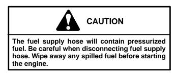
2. Disconnect fuel supply hose from engine fuel rail.
