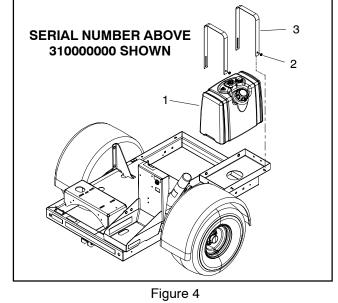
Fuel tank assembly 1. Flange nut (4 used) 2.
