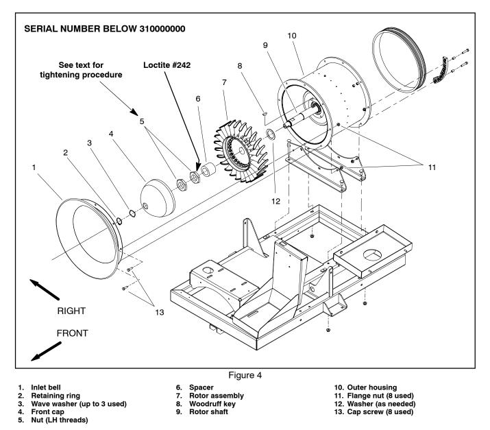
**NOTE:** ProForce blowers with a serial number below 31000000 use two (2) nuts to secure rotor assembly to rotor shaft (Fig. 4). Blowers with serial numbers above 310000000 use one (1) nut (Fig. 5).
