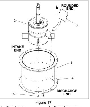
Outer housing Flange head screw 1. 4. Inner housing assembly Flange head screw 2. 5.
