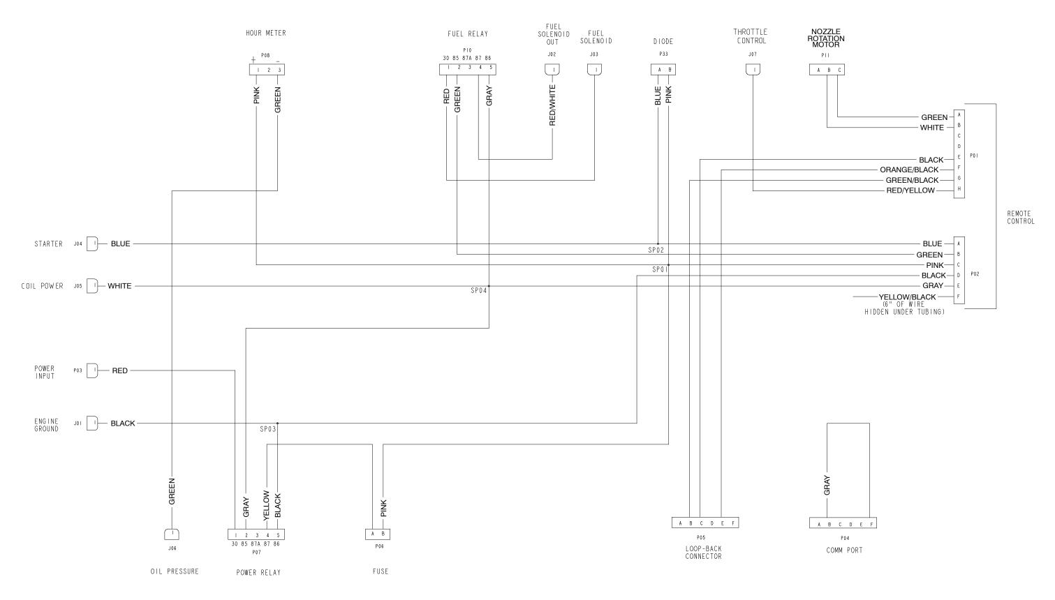
ProForce Debris Blower Model 44538 with Serial Number Below 31000000 Wire Harness Diagram
