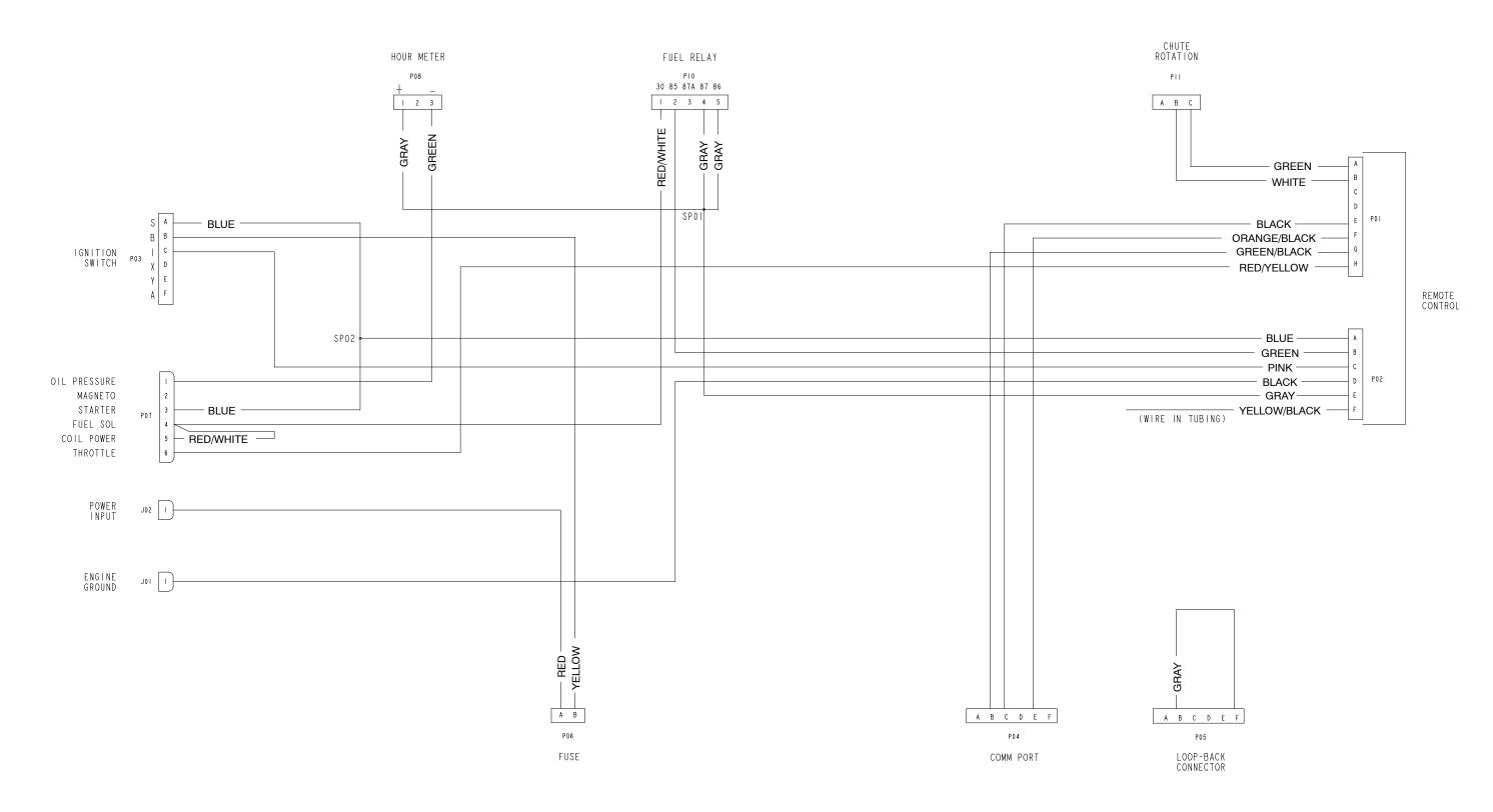
ProForce Debris Blower Models 44538 and 44539 with Serial Number From 310000000 to 311999999 Model 44542 (all Serial Numbers) **Wire Harness Diagram**
