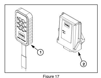
1. Remote transmitter 2. Control module
