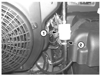
Figure 7 2. Fuel filter inlet
