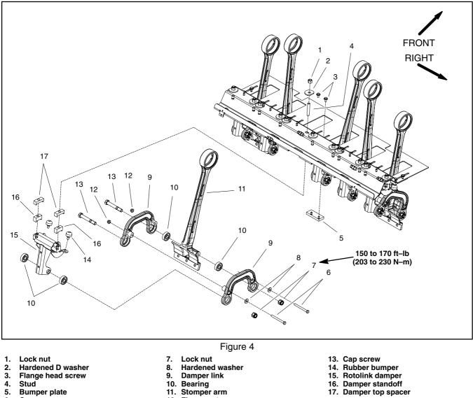
NOTE: The rotolink damper assemblies for all stomper arms used on the ProCore 648 are identical.
