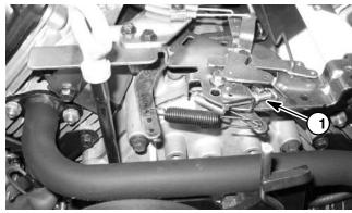
Figure 3 1. High speed screw
