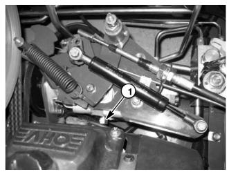
Figure 7 1. By–pass valve location
