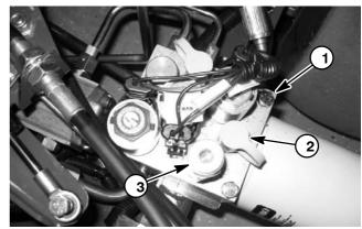
Figure 16 1. Hydraulic manifold 3. Relief valve (R1) G1 port quick fitting
