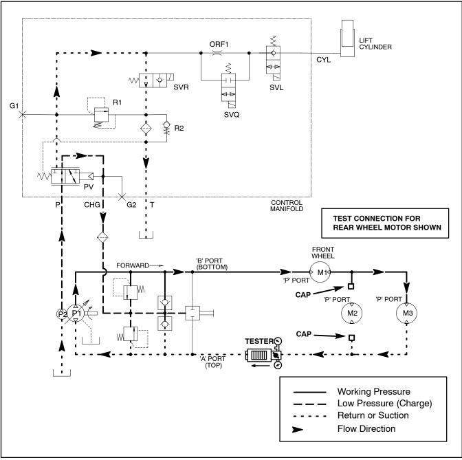
Wheel Motor Efficiency Test (Using Tester With Flow Meter and Pressure Gauge)
