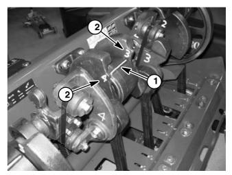
Figure 9 1. Housing timing mark 2. Crankarm position
