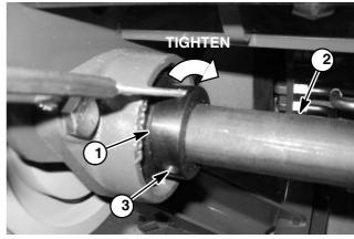
Figure 20 Flange mount bearing 3. Set screw
