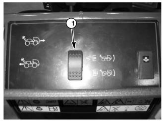
Figure 16 1. Manual raise/lower switch
