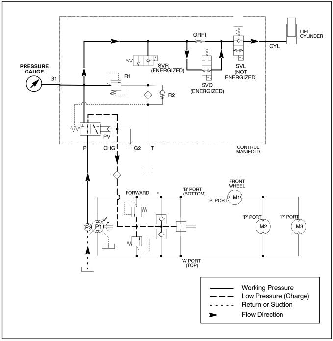
Coring Head Raise/Lower Relief (R1) Pressure Test (Using Pressure Gauge)
