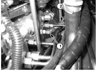
Figure 19 1. Lower 45° fitting 2. Hydraulic hose
