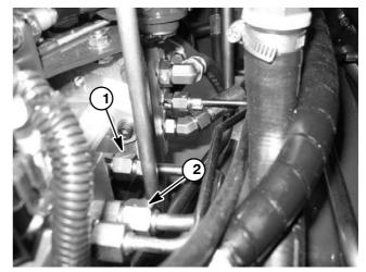
Figure 23 1. Gear pump outlet 2. Manifold port P
