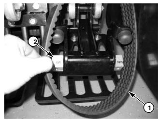
Figure 16 1. Secondary drive belt 2. #1 rotolink damper
