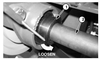
Figure 19 1. Flange mount bearing 2. Jackshaft
