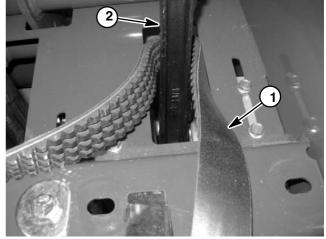
Figure 15 1. Secondary drive belt 2. #1 stomper arm
