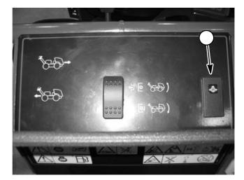
Figure 10 1. Oil pressure indicator light
