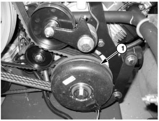
Figure 35 1. Electric clutch
