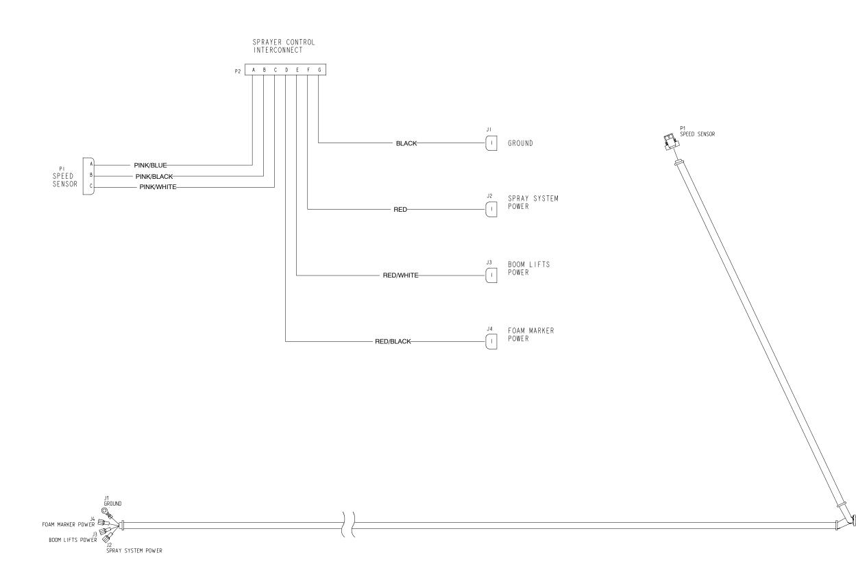
Workman 200 Spray System **Sprayer Power Harness** (Serial Numbers Below 260000000)
