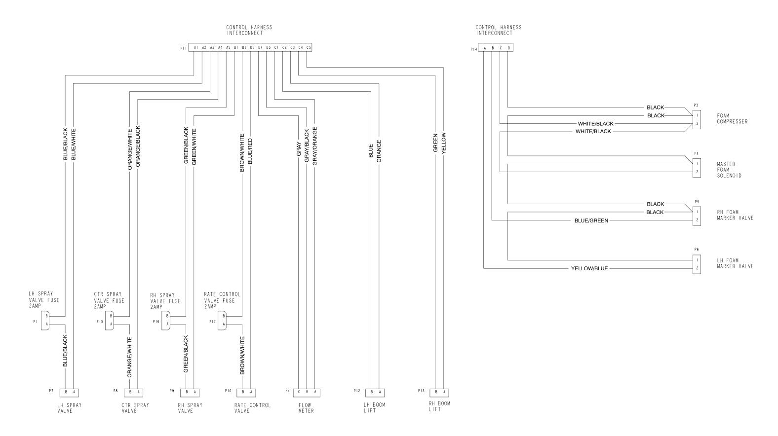
Workman 200 Spray System Spray System Wire Harness (Serial Numbers Below 26000000)
