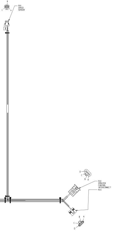
Workman 200 Spray System **Sprayer Power Harness** (Serial Numbers Above 26000000)
