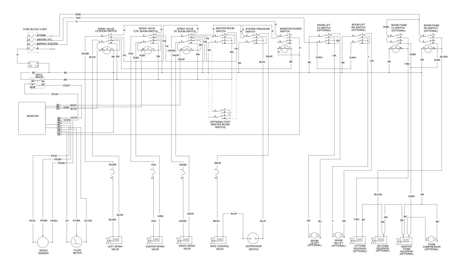
Workman 200 Spray System Electrical Schematic (Serial Numbers Below 26000000)
