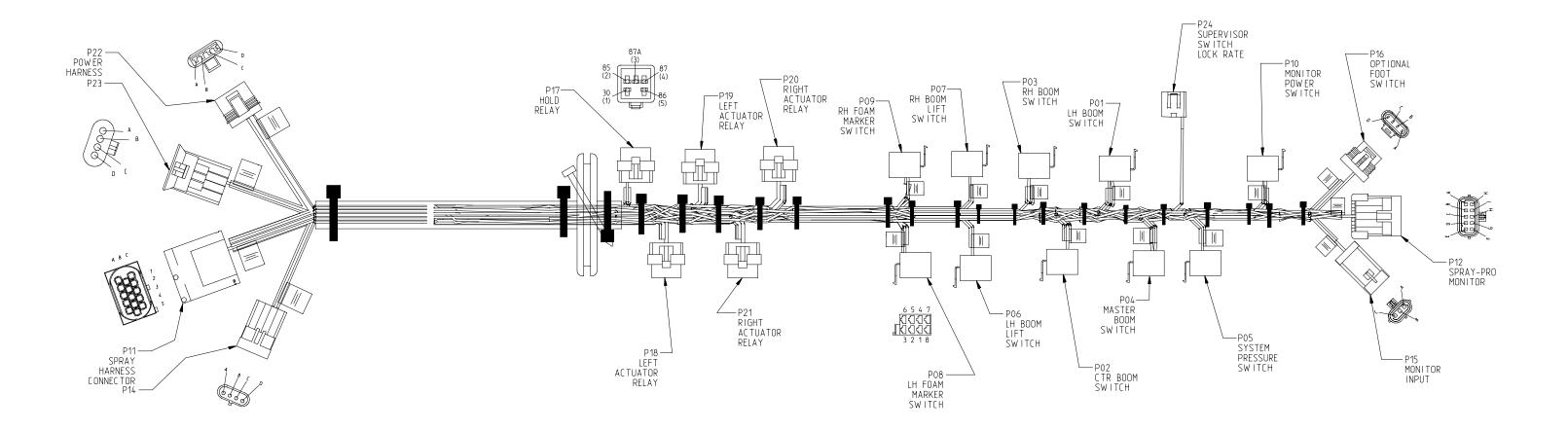
Workman 200 Spray System **Spray Console Wire Harness** (Serial Numbers From 270000001 to 290999999)
