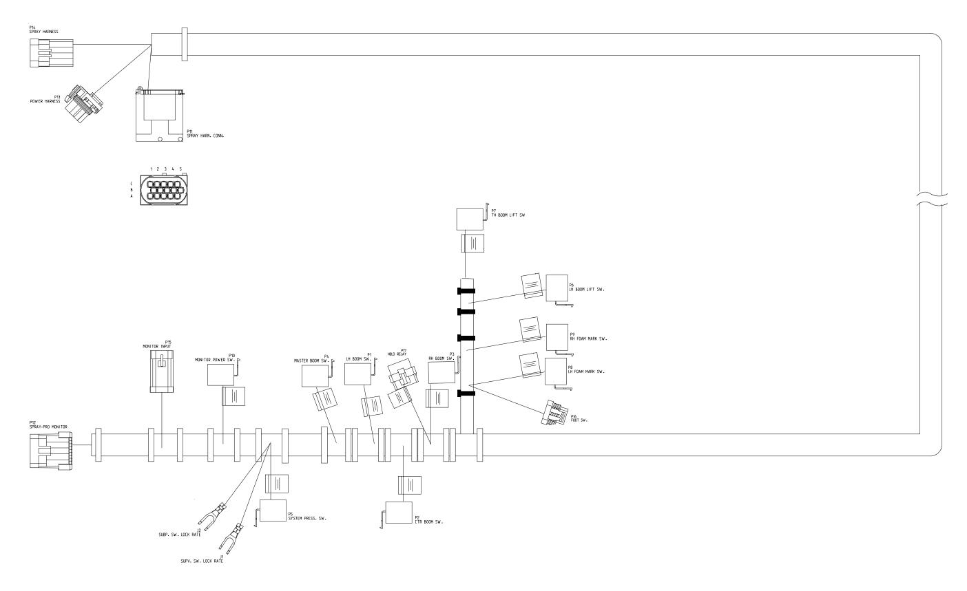
Workman 200 Spray System **Spray Console Wire Harness** (Serial Numbers Below 26000000)
