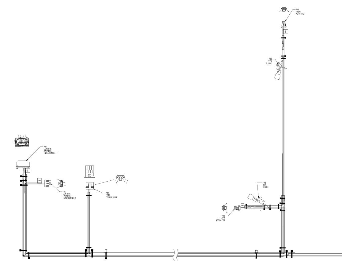
Workman 200 Spray System **Spray System Wire Harness** (Serial Numbers Above 31000000)
