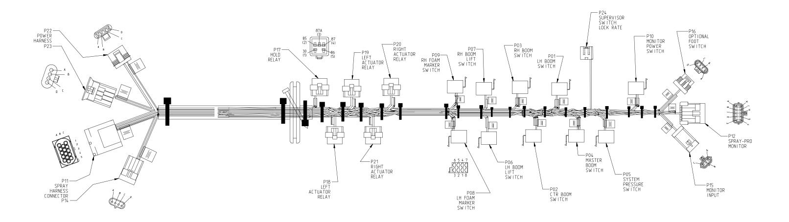
Workman 200 Spray System **Spray Console Wire Harness** (Serial Numbers Above 31000000)
