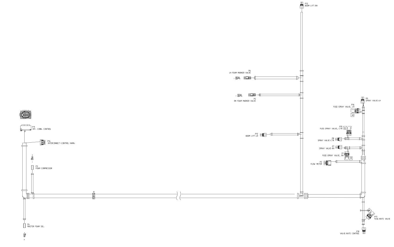
Workman 200 Spray System **Spray System Wire Harness**
