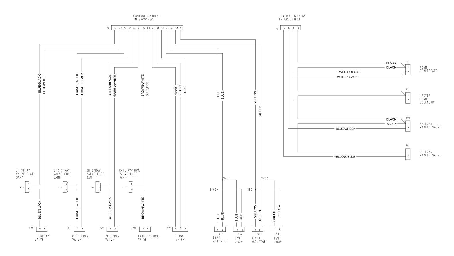
Workman 200 Spray System Spray System Wire Harness (Serial Numbers From 260000001 to 280000200)
