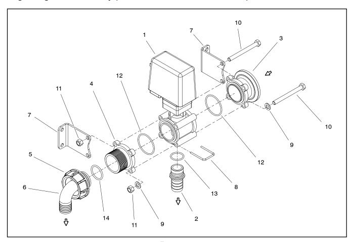
1. Regulating valve motor
