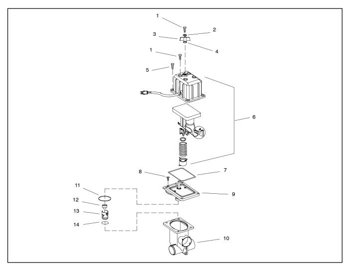
Figure 27 Rate control motor assembly
