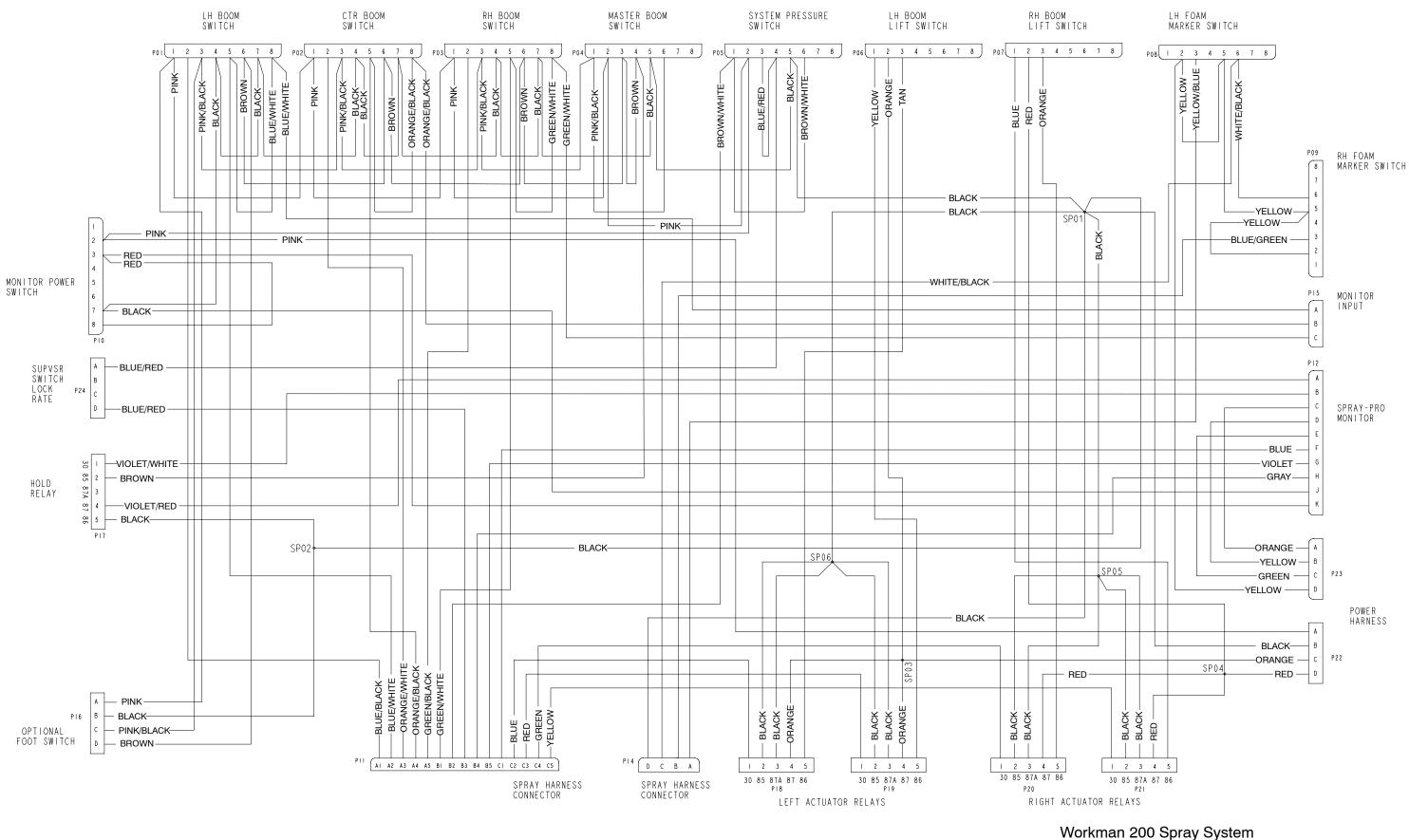
Spray Console Wire Harness (Serial Numbers From 270000001 to 290999999)
