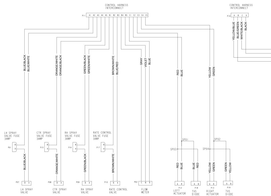
Workman 200 Spray System Spray System Wire Harness (Serial Numbers From 280000201 to 290999999)
