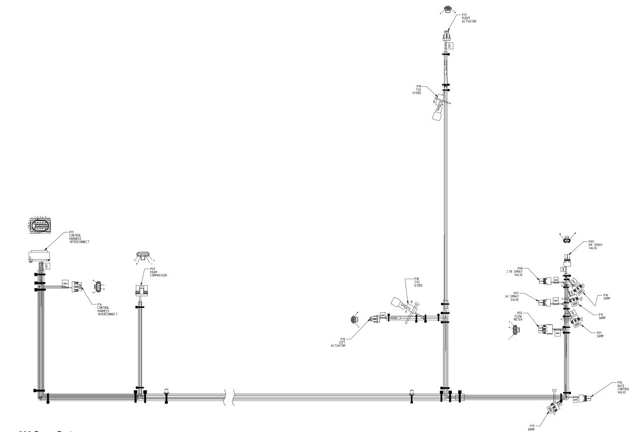
Workman 200 Spray System **Spray System Wire Harness** (Serial Numbers From 280000201 to 290999999)
