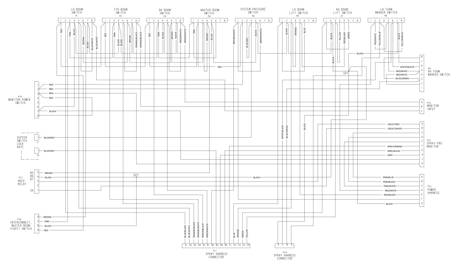
Workman 200 Spray System **Spray Console Wire Harness** (Serial Numbers Below 26000000)
