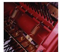
A clean sweep. Nothing cleans turf of leaves and pine needles like the flex tip reel. Its flexible nylon fingers brush the ground clear of debris utilizing a spring-loaded design to give the fingers an extra kick for clearing debris in wet conditions.
