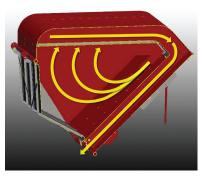
Breathe easy. New air flow system improves dust management and provides a cleaner environment for operator and bystanders.
