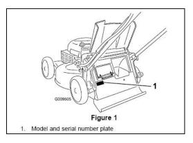
• <u>Toro Super Recycler walk power mowers</u> – the model/serial number can be found on a decal on the left side above the rear wheel of the mower
