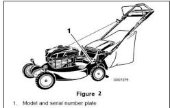
• <u>Toro Commercial 21 walk power mower</u> – the model/serial number can be found on the right side above the rear wheel of the mower
