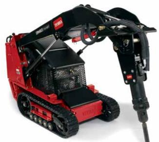
HYDRAULIC BREAKER Horizontal and vertical positions
