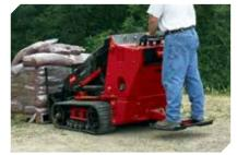
**TX PLATFORM** Allows stand-on operation and folds up for easy walk-behind operation
