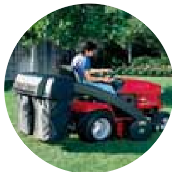
VAC BAGGER Vac bagger develops high vacuum power for collecting. Impeller assembly helps to process debris, so it collects and fills more efficiently for fewer stops.
