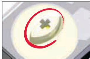
Raised inlets ensure that sediment deposits at the bottom of the tube do not enter the emitter.
