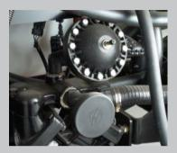
The dual diaphragm pump can be run dry without damage to the seals or pump. The o-ring sealed system components are designed to be leak free and can be disconnected without tools.
