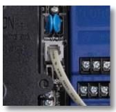
The TriComm Modem Kit connects easily to an installed TMC-424E controller. The data cable for the modem kit plugs into the remote port for the TMC-424E
