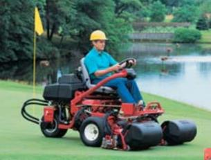
**ENVIED DESIGN** The legendary Toro triplex design, with its unique placement of the cutting units, offers numerous advantages, including the easy-empty center basket. Rear-wheel tracking within the radius of the front wheels helps keep operators out of trouble in sharp turns. The low-mounted engine and hydraulic components provide exceptional hillside stability. This configuration also improves service and maintenance accessibility.
