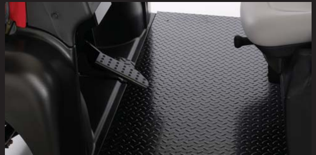
Steel diamond plate floorboards provide a rugged appearance and a durable surface.
