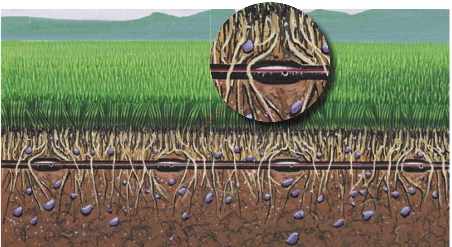
DL2000 with ROOTGUARD protection inhibits root intrusion directly at the emitter opening.
