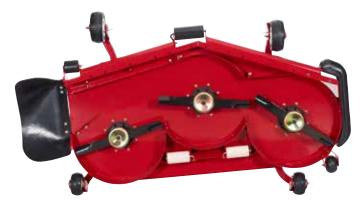
Side Discharge Decks – The patent pending adjustable front baffle allows you to fine tune the deck performance to meet changing turf conditions. The baffle position adjusts in a matter of seconds with no tools required. The patent pending rubber discharge deflector disperses clippings evenly while protecting tree bark from damage.
