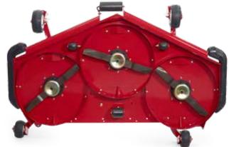
Guardian Recycler Decks – A patented vertical discharge system offers improved safety and clipping management by forcing clippings to be cut and re-cut. Recycler decks can be easily converted to rear discharge with optional kit for added versatility.
