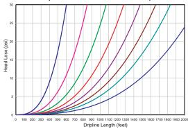
Head Loss v. Dripline Length and Emitter Spacing Drip In 20mm .63 GPH PC Emitter 0% Slope.
