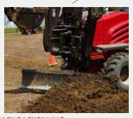
EASY BACKFILLING. Six-way heavy-duty backfill blade is standard. The float position allows blade to smoothly follow the ground's contours.
