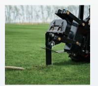
**CONSISTENT PLOWING** Optimized plow design provides down pressure to maintain consistent plowing up to 24" deep in a variety of conditions. The 10-degree frame oscillation ensures constant wheel-to-ground contact when plowing over rough terrain or crossing open trench lines.
