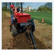
**PRODUCTIVE TRENCHING** with optional front-mounted, hydraulically-driven trencher. Dig depths of 24" or 36" (61 cm or 91 cm).
