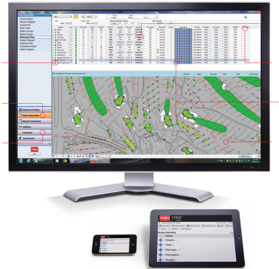
Lynx Mobile Enables remote access and control from any mobile device connected to the Internet. Screens are specifically designed and optimized for smaller devices.
