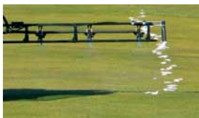
Pro Foam Marking Kit - 41236: Foam dollops ensure accurate parallel path tracking. Select foam for either boom or both.
