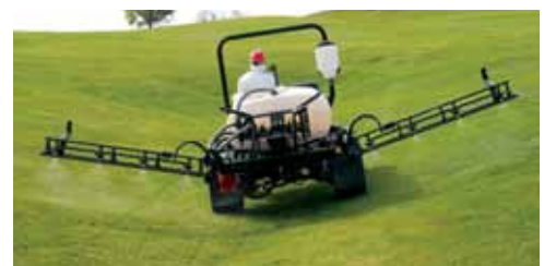
Ultra Sonic Boom Leveling Kit - 41218: New sonar sensors attached to end of the booms automatically maintain proper spray height over undulating turf.
