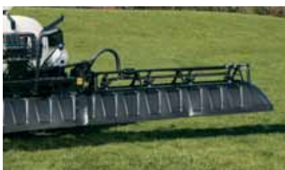
Drift Reduction Boom Shroud Kit - 41602: Reduces spray drift in windy conditions.
