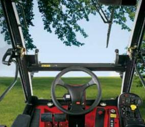
The Groundsmaster 4010-D and 4110-D feature a climate-controlled safety cab, with rollover protection and a pressurized air filtration system that keeps dust and debris away from the operator.
