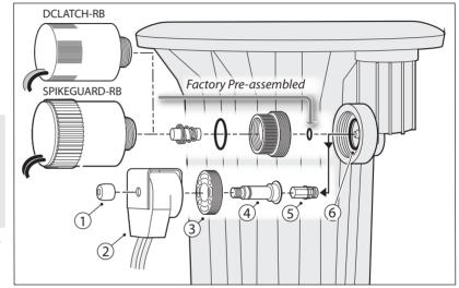
2. Unscrew and remove the plunger assembly retainer (3) using a Rain Bird universal sprinkler tool or needle-nose pliers. Remove the plunger assembly, comprised of plunger shaft (4) and plunger (5).
